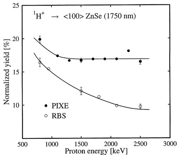
Fig. 2. The experimental RBS and PIXE minimum yields vs. incident proton energy from a 1750 nm thick ZnSe sample. The beam angular divergence was  $0.015^\circ$ . Solid lines were drawn to guide the eye.
