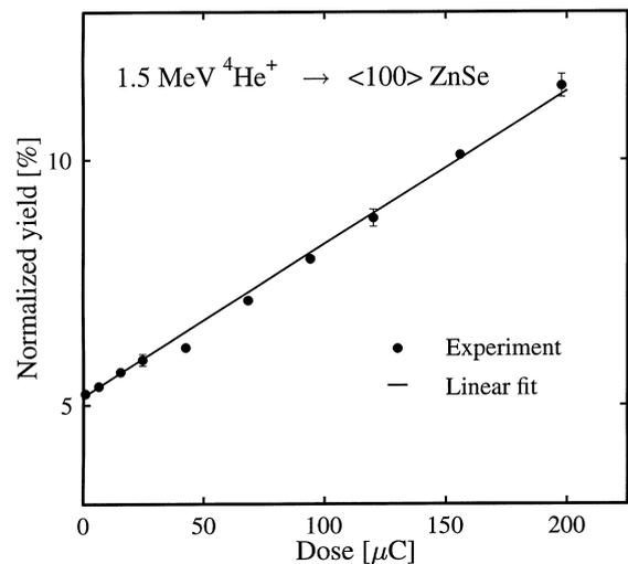
Fig. 1. The RBS minimum yield of  $^4\text{He}$  ions incident on a ZnSe sample as a function of accumulated ion dose. The irradiations were done with 1.5 MeV  $^4\text{He}$  ions with the sample aligned along the  $\langle 100 \rangle$  crystallographic axis.
