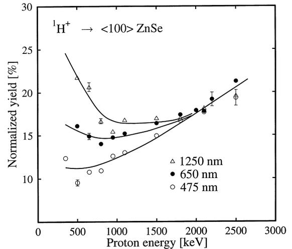
Fig. 5. The experimental PIXE minimum yield vs. incident proton energy from ZnSe samples with thicknesses of 475, 650 and 1250 nm. The beam angular divergence was  $0.030^\circ$ . Solid lines as in Fig. 2.
