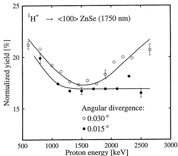
Fig. 3. The experimental PIXE minimum yields vs. incident proton energy from a 1750 nm thick ZnSe sample with beam angular divergences of  $0.015^\circ$  and  $0.030^\circ$ . Solid lines as in Fig. 2.
