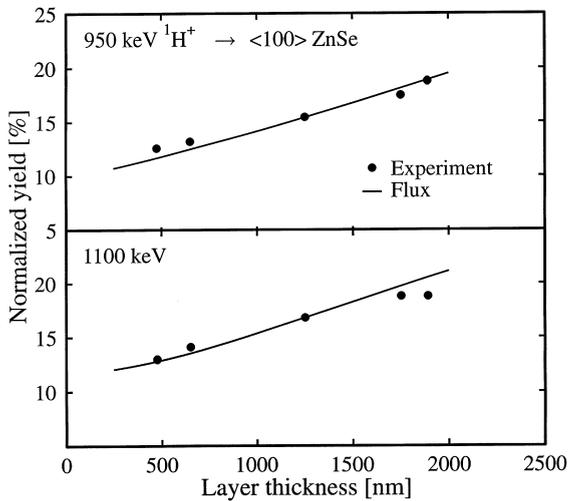
Fig. 4. The PIXE minimum yield vs. ZnSe layer thickness measured with proton energies of 950 and 1100 keV. The beam angular divergence was  $0.030^\circ$ . The experimental values are indicated by the points and the lines represent the values simulated with the code Flux. In this figure the statistical uncertainty of the experimental values is within the size of the symbols due to the scale of the  $y$ -axis.
