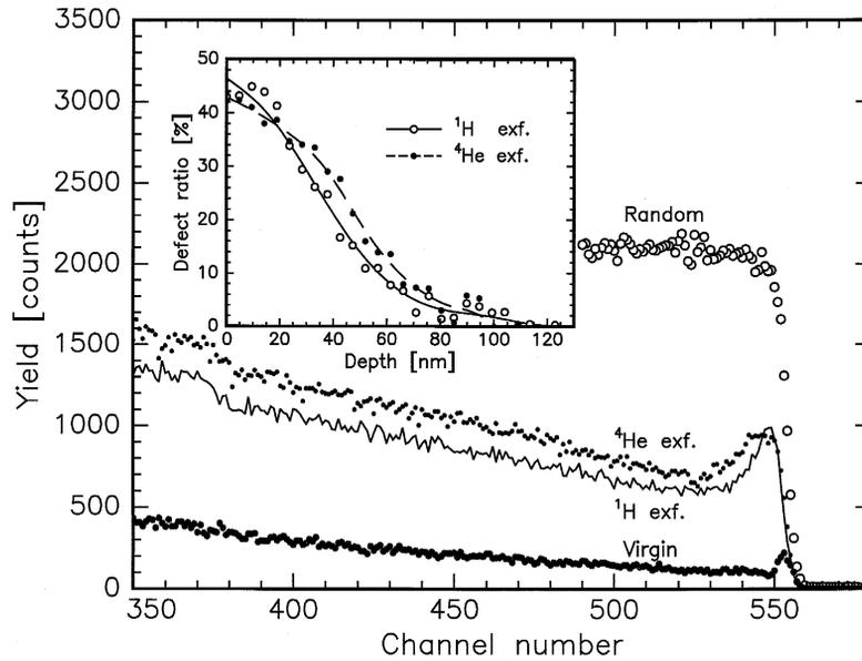
Fig. 2. Random and channelling spectra ( $\langle 100 \rangle$  axial direction) obtained from the bottom of  $^1\text{H}$  and  $^4\text{He}$  induced craters by 2.0 MeV  $^4\text{He}$  Rutherford backscattering. In the insert, the deduced defect distributions are shown for the 0.6 MeV  $^1\text{H}$  and 1.4 MeV  $^4\text{He}$  ion implanted InP.
