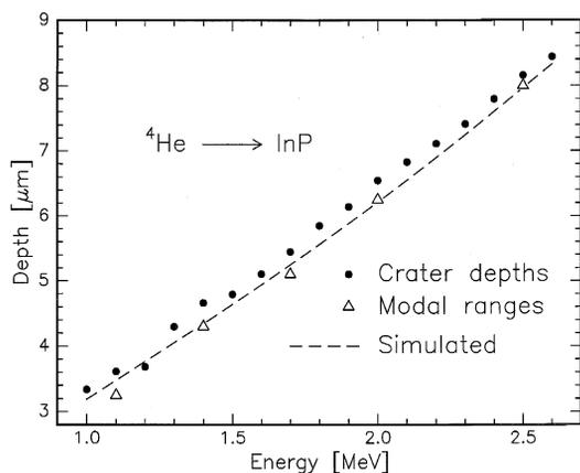
Fig. 3. The measured modal  $^4\text{He}$  ion ranges and crater depths in InP. Simulated range values were obtained by Monte Carlo calculations.
