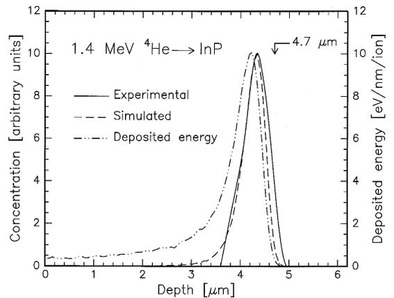
Fig. 1. Depth distribution of 1.4 MeV  $^4\text{He}$  ions implanted in InP at random orientation. The experimental profile is shown by the solid line. The corresponding measured crater depth is indicated by the arrow. The simulated range (dashed) and deposited energy distributions (dashdotted curve) are from Monte Carlo calculations.
