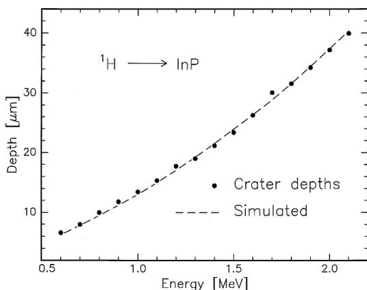
Fig. 4. The crater depths produced in InP by proton bombardment and the corresponding simulated modal range values obtained by Monte Carlo calculations.
