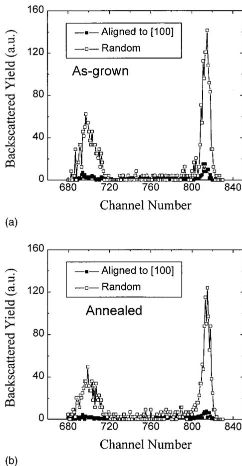
FIG. 2. Nuclear reaction yields as a function of energy (shown as channel number) obtained for a random direction and aligned to [100] from: (a) as-grown and (b) annealed  $\text{GaN}_{0.03}\text{As}_{0.97}$  epilayer grown by GSMBE.
