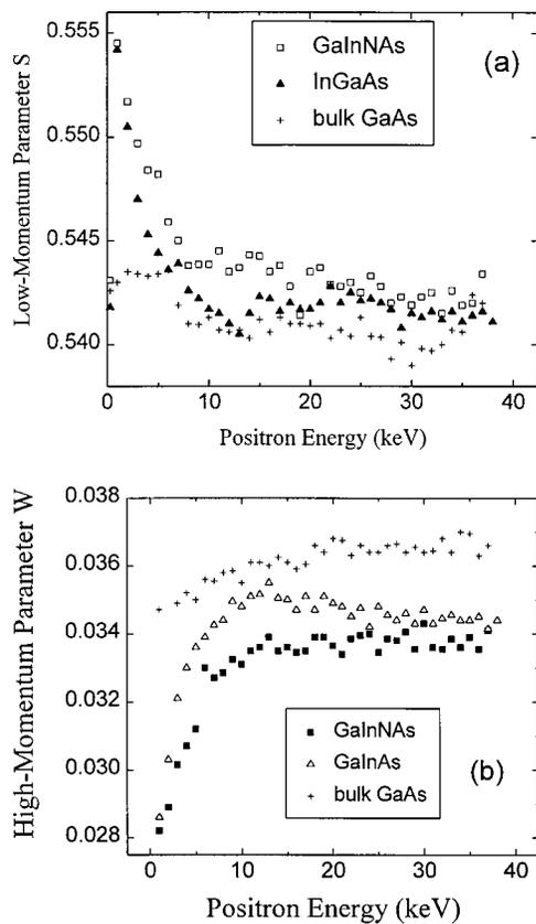
FIG. 1. (a) Low-momentum parameters  $S$  and (b) high-momentum parameter  $W$  as a function of positron incident energy in as-grown  $\text{Ga}_{0.94}\text{In}_{0.06}\text{N}_{0.02}\text{As}_{0.98}$  sample. For comparison, the data for a bulk GaAs (defect free) and a  $\text{Ga}_{0.99}\text{In}_{0.01}\text{As}$  sample grown under the same condition are also shown.
