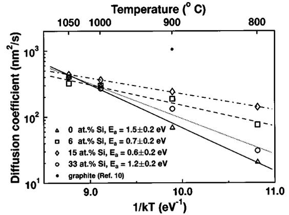
FIG. 5. Arrhenius plot for the diffusion coefficient of non-trapped deuterium. Shown are the natural logarithms of the diffusion coefficients vs  $1/kT$ . The lines are the fits to the experimental data.
