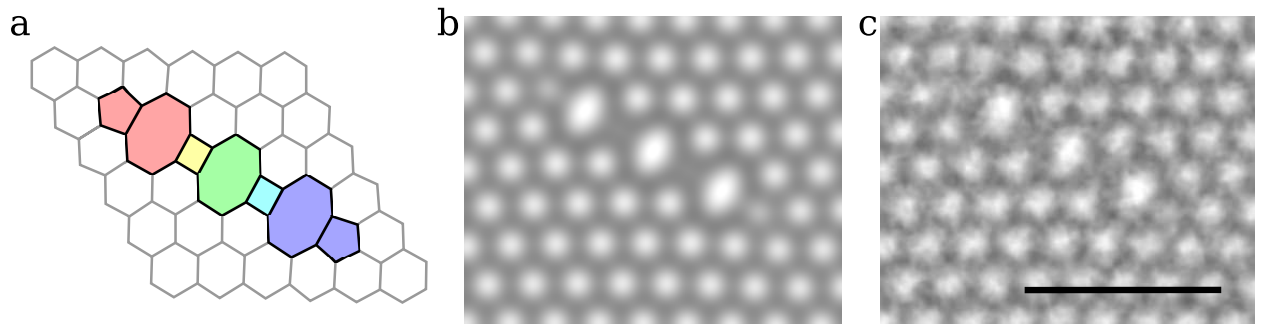
Figure 2: DFT-optimized structure of the defect with two tetragons (a), HRTEM simulation based on the DFT-structure (b) and the HRTEM image of the same structure for comparison (c). Scale bar is 1 nm.
